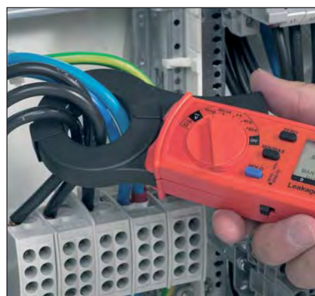
Differential current measurement with leakage current clamp
