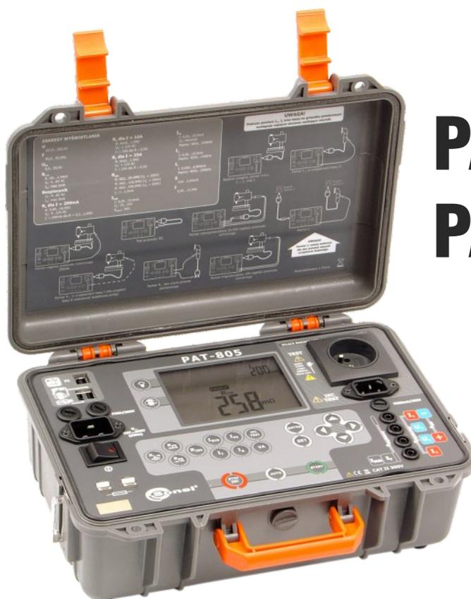
PAT-800 and PAT-805 digital meters are used to measure the parameters of portable electrical equipment (power tools, white goods, etc.) which determine their safety: **resistance of protective conductors, insulation resistance, continuity of connections, leakage current, power.**
